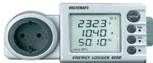
Figure 2. Voltcraft Energy Logger 4000 (Photo Credit: Voltcraft.com)
